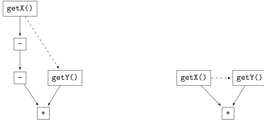
Figure 11: The sea-of-nodes graph for -(-x)+y Figure 12: The optimized sea-of-nodes graph
